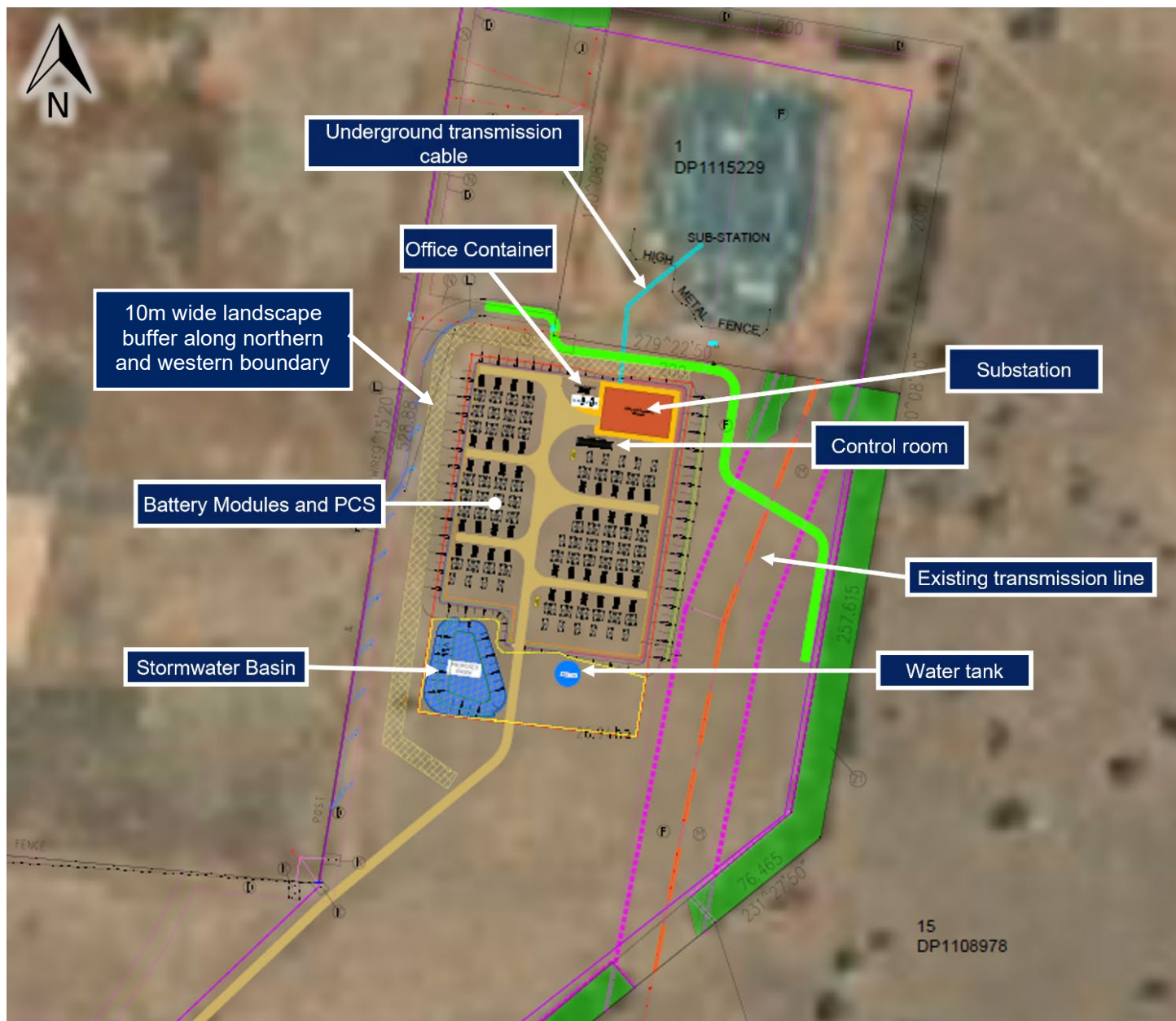
Figure 5 | BESS Infrastructure Site Layout
