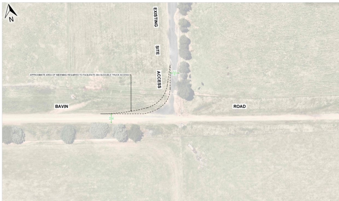
Figure 9 | Site Access Widening
